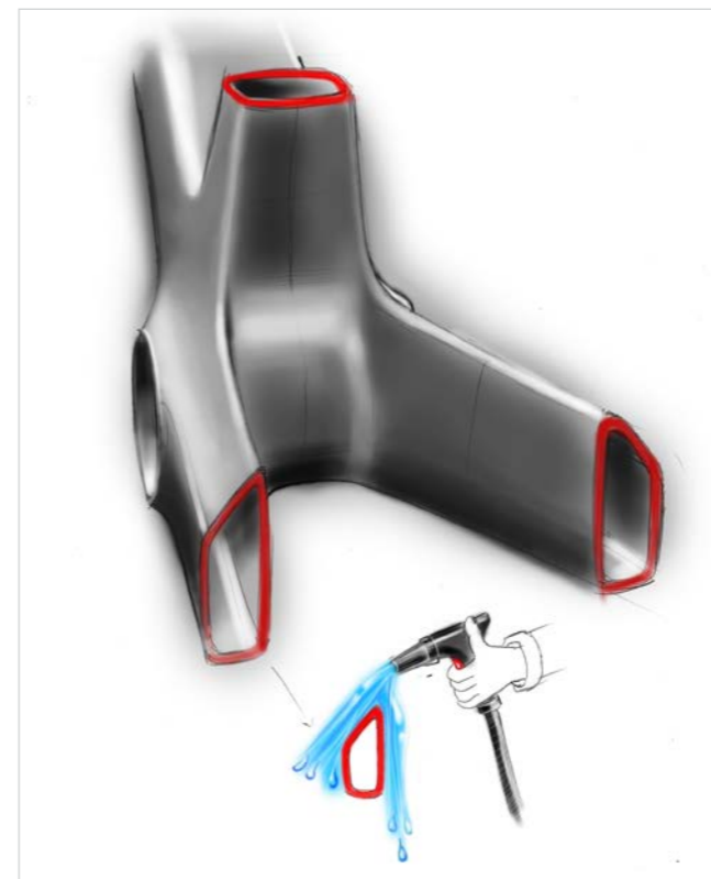
From concept to reality: mud-shedding chainstays
