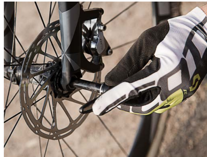
Thru-axle allow for an easy installation of disc brake wheels
