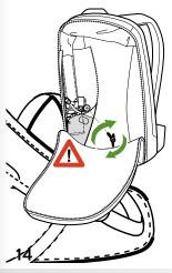
TURN THE SCREW TO LOAD THE INFLATOR SYSTEM AND UNSCREW TO REMOVE TOOL.
