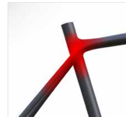
A direct connection between toptube and seat stays increases vertical compliance
