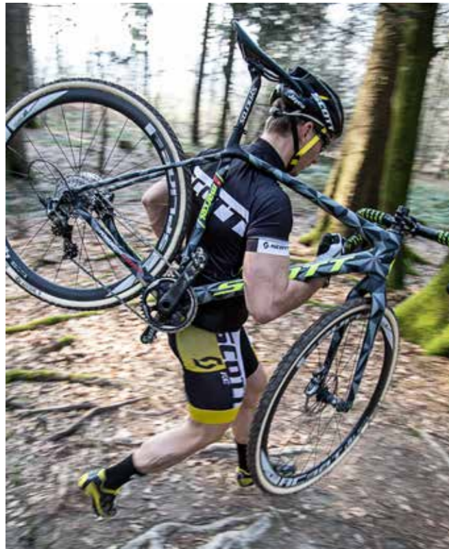
Ergonomic tube shapes facilitate carrying the bike
