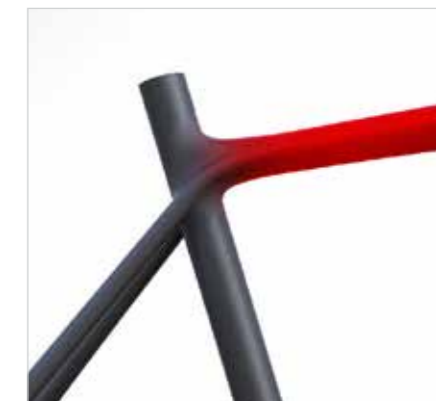
The toptube becomes more oval towards the connection with the seattube
