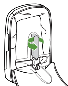
STEP 14 Unscrew the cartridges.
